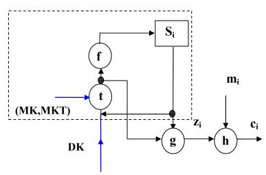
Figure 1. Model of the HENKOS stream cipher
