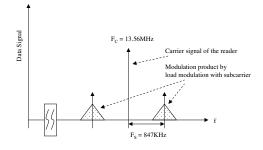
Fig. 11. Load Modulation - side band.
