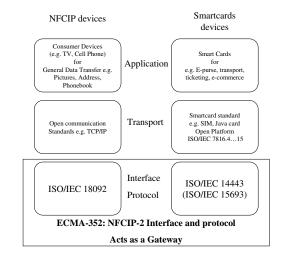
Fig. 2. NFCIP devices vs. Smartcards devices.
