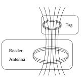
Fig. 10. Near Field Communication via Inductive coupling.
