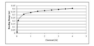
Fig. 5. Leech-to-Card distance as a function of current.
