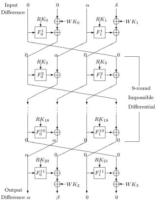
Fig. 4 Impossible Differential Attack on 11-round CLEFIA (2)
