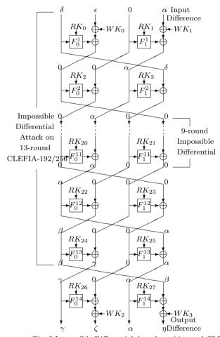
Fig. 5 Impossible Differential Attack on 14-round CLEFIA-256  $\,$
