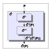
**Fig. 2.** Cascade obfuscator  $\mathcal{O}$  receives a program P, and applies  $\mathcal{O}'$  and  $\mathcal{O}''$  sequentially. The resulting obfuscated program  $\mathcal{O}''(\mathcal{O}'(P))$  is then output.
