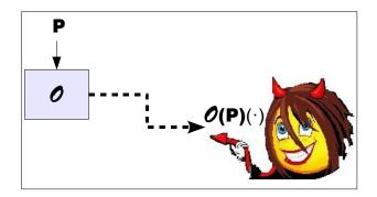
**Fig. 4.** A program P is obfuscated, and then sent to remote platform. The user controlling the execution environment can execute the obfuscated program on any input of its choice and can observe the outputs. The virtual black-box property requires that the user does not learn more about the program than an oracle access to the program would reveal.
