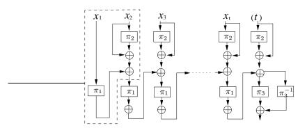
Fig. 7. The enhanced three-key enciphered CBC mode
