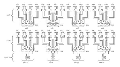
Fig. 2. Optimized architecture with Four-Nibbles bundle path.
