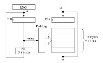
Fig. 5. RNG processing Architecture.
