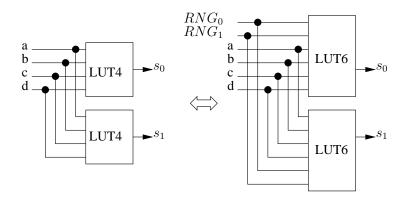
Fig. 3. Using two RNG pins does not add ALMs.
