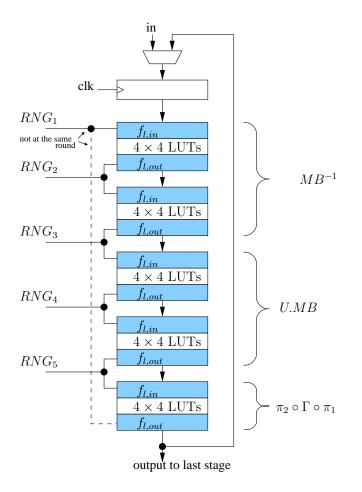
Fig. 4. Architecture with 5 layers of LUTs.
