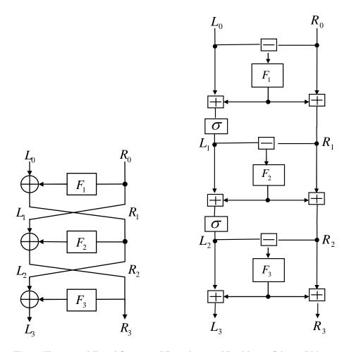
Fig. 1. The 3-round Feistel Structure  $LR_3$  and 3-round Lai-Massey Scheme  $LM_3$ .
