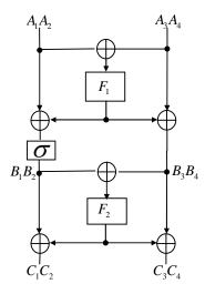
**Fig. 2.** Two-round FOX-style Lai-Massey Scheme.  $\sigma(x, y) = (y, x \oplus y), \oplus$  means the bitwise exclusive or operation(xor).
