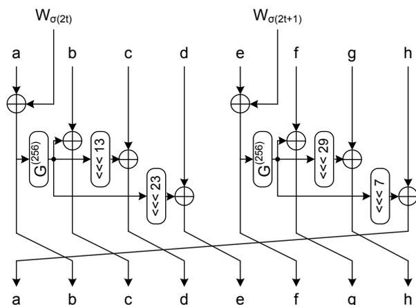
Figure 2. Step function of ARIRANG-256 for round  $t$ .
