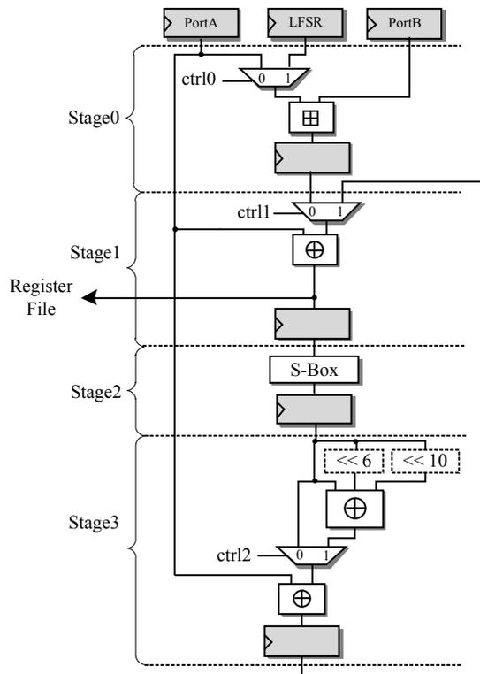
**Figure 6.** Datapath of the Coprocessor for Hummingbird.
