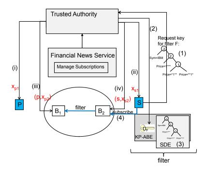
Fig. 4. Key and message exchange for filter generation.
