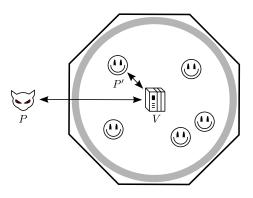
Figure 3: Real-world scenario for Distance Hijacking. P has a (stolen) smartcard. However, he cannot enter the secure facility and he does not have any collaborators inside the facility. In a Distance Hijacking attack, P exploits the presence of an honest P' to convince V that P is within the secure facility.
