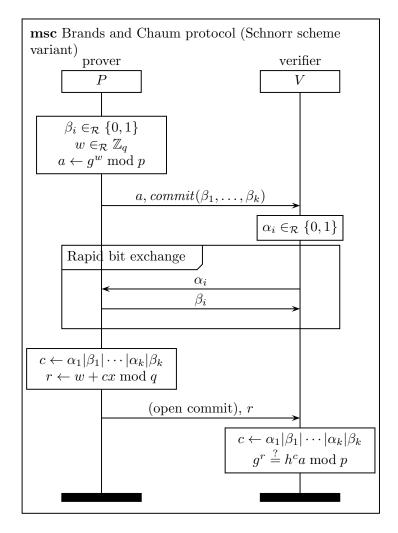
Figure 16: Brands and Chaum protocol based on the Schnorr identification scheme. The public key of the prover is the tuple  $(p, q, g, h = g^x \mod p)$  and the corresponding private key is x.
