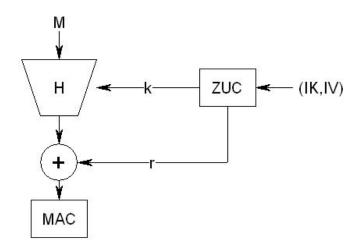
Fig. 1. Structure of 128-EIA3
