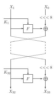
Fig. 1. Encryption procedure of LBlock
