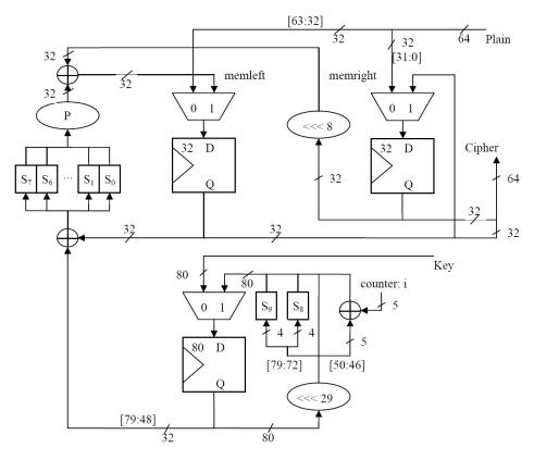
${\bf Fig.\,3.}$  The data path of an area-optimized version of LBlock
