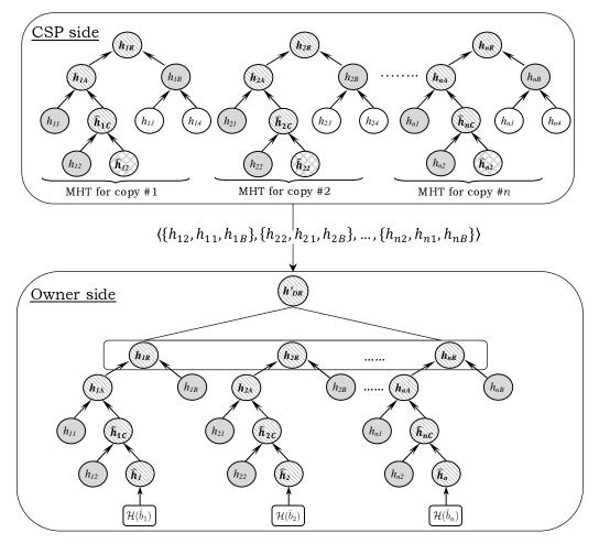
Fig. 14: Effect of block insertion operation on the MHTs and the directory root.
