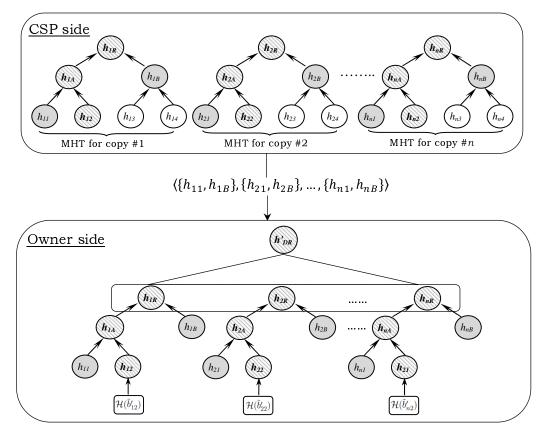
Fig. 13: Effect of block modification operation on the MHTs and the directory root.
