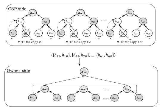
Fig. 15: Effect of block deletion operation on the MHTs and the directory root.
