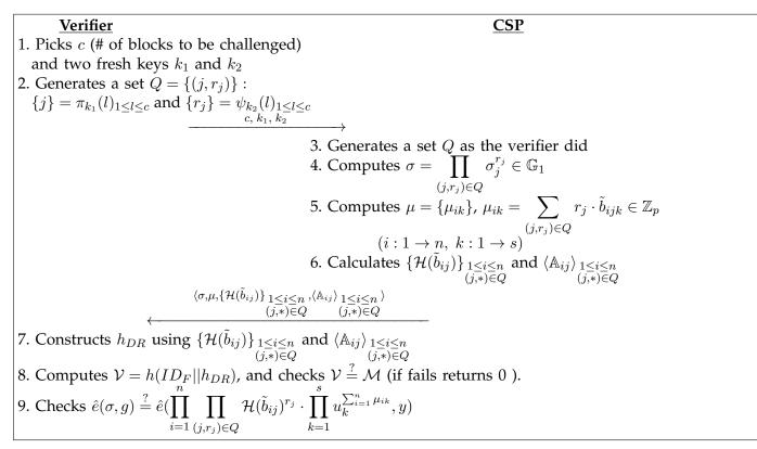
Fig. 9: The challenge response protocol in the TB-DMCPDP scheme
