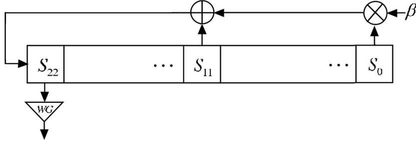
Fig. 1. The WG-7 Stream Cipher Scheme
