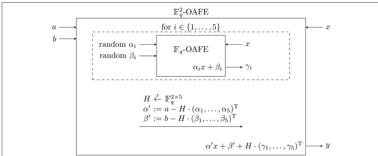
Figure 9: Implementation of  $\mathbb{F}_q^2$ -OAFE from five instances of  $\mathbb{F}_q$ -OAFE; protocol taken from [DKMQ12]. Additional measures must be taken so that  $H$  is not announced before the receiver party has provided some input to all five underlying  $\mathbb{F}_q$ -OAFE instances in the dashed box; otherwise the protocol is inherently insecure, as shown in [DKMQ12, Lemma 1].
