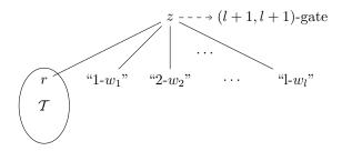
Figure 2: The tree  $\mathcal{T}_w$ , where "1- $w_1$ ", "2- $w_2$ ",  $\cdots$ , "l- $w_l$ " are components of a prefix  $w = w_1 w_2 \cdots w_l$   $(1 \le l \le d)$  of some time period. The time period is d-bit long.
