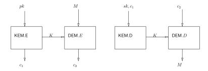
Figure 1: Hybrid encryption with a KEM/DEM construction. The left side shows the encryption operation, and the right side shows the decryption operation.
