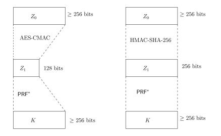
Figure 5: Extract-then-expand KDFs for ECC at the 128-bit security level. On the left the extract function is AES-CMAC and on the right it is HMAC-SHA-256. The choice of PRF<sup>\*</sup> is not important for this our example.
