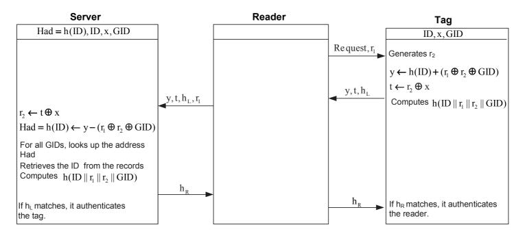
Fig. 2. SUAP2 authentication protocol proposed by Morshed et al. [8].
