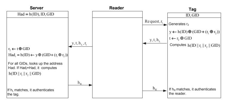
Fig. 3. SUAP3 authentication protocol proposed by Morshed et al. [8].
