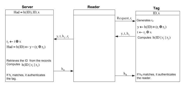
Fig. 1. SUAP1 authentication protocol proposed by Morshed et al. [8].
