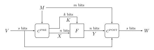
Fig. 1. General compression function of (m + s) to s bits. In [32], F is a blockcipher with a k-bit key, while in [6] F is an unkeyed permutation with n = s.
