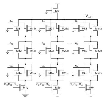
Figure 2: Circuit schematic of the 2D subthreshold current array.
