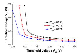
Figure 3: Response nonlinearity in the single-row array: nonlinearity of additive subthreshold current behavior.
