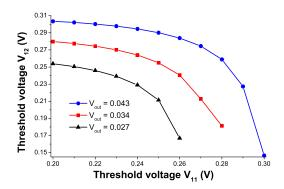
**Figure 4:** Response nonlinearity in the single-column array: nonlinearity of series-connected subthreshold FETs.
