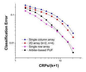
${\bf Figure~8:~} {\it Classification~error~from~modeling~an~8-bit~PUF~via~an~SVM-based~attack}.$
