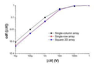
**Figure 10:** Cumulative distribution of  $|\Delta V|$  for three array topologies.
