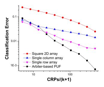
Figure 9: Classification error from modeling a 16-bit PUF via an SVM-based attack.
