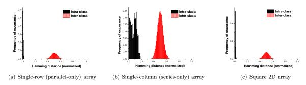
Figure 6: Inter-class and intra-class HD for three array topologies.
