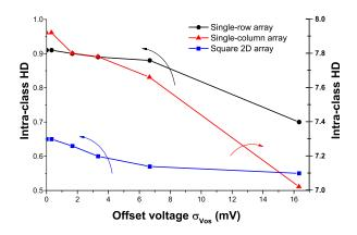
Figure 11: Dependence of intra-class HD on offset voltage spread.
