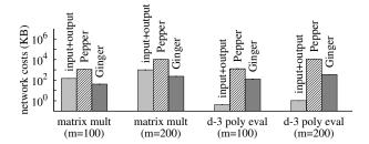
Figure 6—Per-instance network costs of GINGER and its base (PEPPER [48]), compared to the size of the inputs and outputs. At this batch size ( $\beta=5000$ ), GINGER's refinements reduce per-instance network costs by a factor of 20–30 compared to PEPPER. GINGER's network costs here are hundreds of KB or less. The y-axis is log-scaled.
