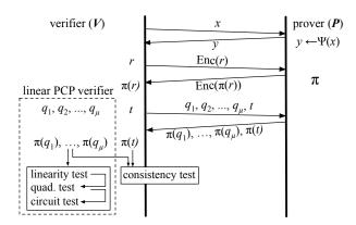
Figure 1—The PEPPER protocol [48], which is GINGER's base. Though not depicted, many of the protocol steps happen in parallel, to facilitate batching.
