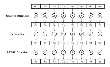
**Fig. 3.** The bijective function F of TCS\_SHA-3-256; S, T and L are 32-bit to 32-bit functions
