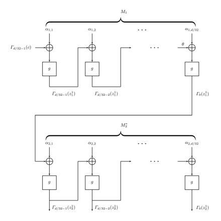
**Fig. 5.** Round 1 of TCS\_SHA-3 (k=2) with 32-bit cipher block chaining;  $\alpha_{1,j} = \Gamma_{d/32-j}(M_1)$  and  $\alpha_{2,j} = \Gamma_{d/32-j}(M_2^*)$ , for all  $j \in \{1, 2, ..., d/32\}$
