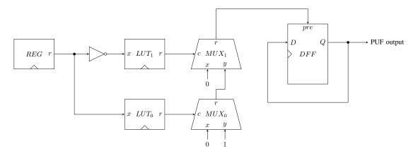
Figure 2: The Anderson PUF design, which realises the first (i.e., sampling) step in Figure 1 (note that clock signals driving REG,  $LUT_0$ ,  $LUT_1$  and DFF are omitted for clarity).
