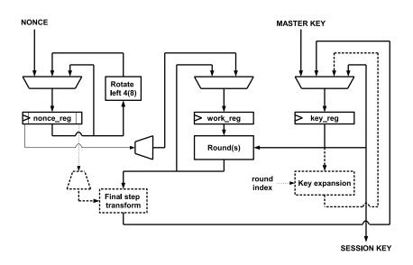
Fig. 6. Overview of our open source hardware architecture for fresh re-keying.
