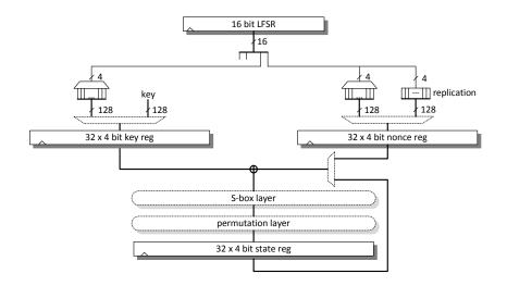
Fig. 7. Prototype architecture for worst-case EM profiling.
