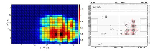
**Fig. 5.** Left: SNR over the  $27 \times 27$  chip surface. Right: Placement on the floorplan
