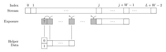
Fig. 7. Snake I helper data, illustrated for a single round. Newly exposed bits are shaded.
