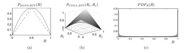
**Fig. 4.** (a) Probability of a response bit mismatch. The dashed curve corresponds with a majority vote during enrollment, in the ideal case. (b) Probability of a response bit collision. (c) Probability density function of R for our 65nm PUF.
