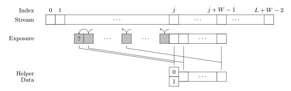
Fig. 9. Snake II helper data, illustrated for a single round. Newly exposed bits are shaded.
