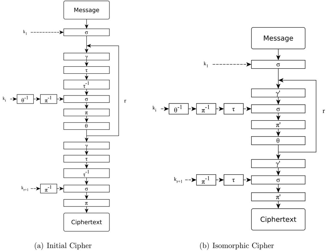
Figure 5: Modified AES with an Invertible Linear Function
