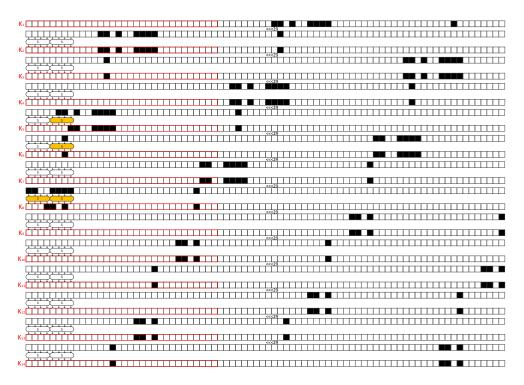
Fig. 2: A 14-round Related-key Differential Characteristic of LBlock (Characteristic in the Key Schedule Algorithm); a black square represents 1, and a white square represents 0.
