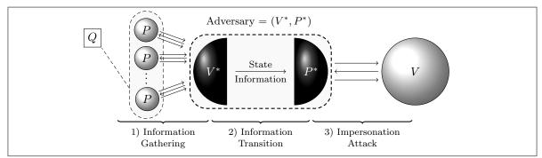
Figure 1: The smart-card authentication model.
