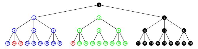
Figure 3: The subset cover  $S_c$  for  $\mathcal{R} = \{14, 15, 22\}$  will contain the SD subsets  $S_{1,\{14,15\}}$ ,  $S_{2,\{22\}}$  and  $S_{0,\{1,2\}}$ .
