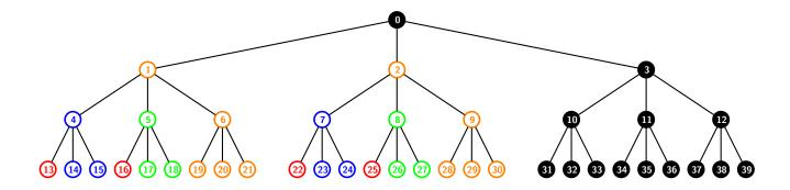
Figure 4: Example showing that the upper bound of 2r-1 on the header length is tight for k=3. The subset cover for  $\mathcal{R} = \{13, 16, 22, 25\}$  in the tree  $\mathcal{T}^0$  with k=3, will contain the SD subsets  $S_{4,\{13\}}$ ,  $S_{5,\{16\}}$ ,  $S_{7,\{22\}}$ ,  $S_{8,\{25\}}$ ,  $S_{1,\{4,5\}}$ ,  $S_{2,\{7,8\}}$  and  $S_{0,\{1,2\}}$ .
