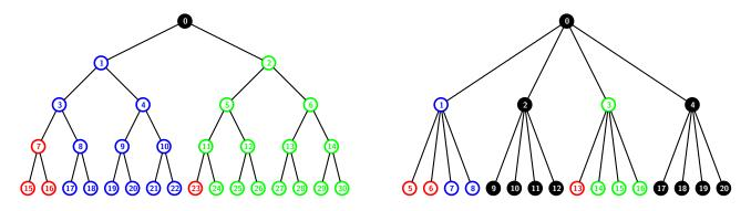
Figure 6: Example where the header length of 2-ary is better than 4-ary: For n=16 users, the header length for  $\mathcal{R}=\{15,16,23\}$  in the 2-ary tree is more for k=4 than for k=2. For k=2, the subset cover  $S_c=\{S_{1,\{7\}},S_{2,\{23\}}\}$ . For k=4, the subset cover  $S_c=\{S_{1,\{5,6\}},S_{3,\{13\}},S_{0,\{1,3\}}\}$ .
