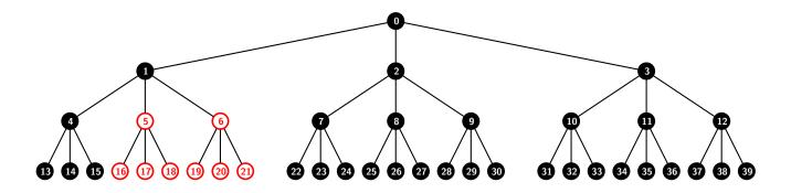
Figure 1: The k-ary tree  $\mathcal{T}^0$  with k=3 and n=27 users. The subset  $S_{0,\{5,6\}}$  contains all users (leaves) in the subtree  $\mathcal{T}^0$  but not in  $\mathcal{T}^5$  or  $\mathcal{T}^6$ . Hence,  $S_{0,\{5,6\}} = \{13,14,15,22,23,\ldots,39\}$ .
