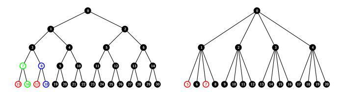
Figure 5: Example where the header length of 4-ary is better than 2-ary: For n=16 users, the header length for  $\mathcal{R}=\{15,17\}$  in the 2-ary tree is more for k=2 than for k=4. For k=2, the subset cover  $S_c=\{S_{7,\{15\}},S_{8,\{17\}},S_{0,\{3\}}\}$ . For k=4, the subset cover  $S_c=\{S_{0,\{5,7\}}\}$ .
