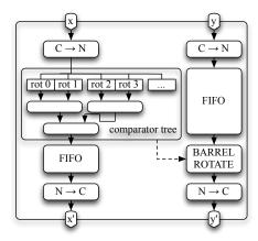
Fig. 2. Simplified point addition module. The grey shaded blocks are without registers.
