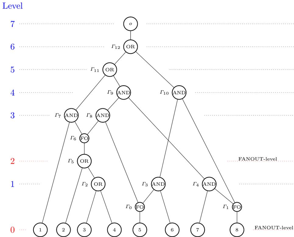
**Fig. 1.** Boolean circuit with FANOUT-gates
