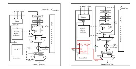
Fig. 5. AES architecture without Trojans Fig. 6. AES architecture with Trojan 1
