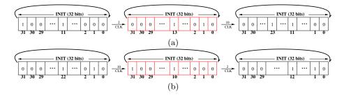
Fig. 7. Operations of CFGLUT5 to activate the Trojan and restore to normal operations for (a) Trojan 1; (b) Trojan 2. Bit positions not shown contain '0'
