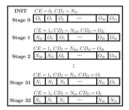
Fig. 2. INIT value reconfiguration in CFGLUT5
