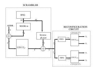
Fig. 10. Architecture of Sbox Scrambler
