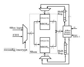
Fig. 8. Architecture of Sbox Computation using affine transformation and storing in RLUT  $\,$
