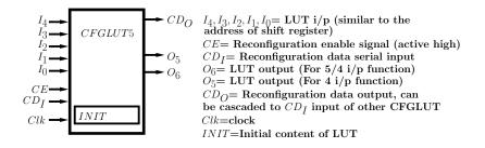
Fig. 1. Block diagram of CFGLUT5
