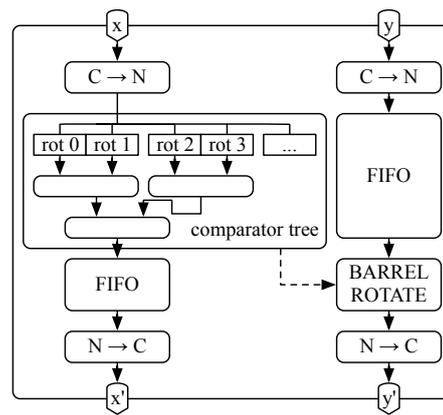
**Fig. 5** Point automorphism unit with  $m$  comparator units.
