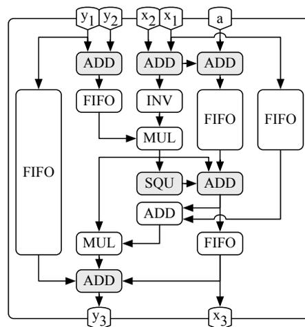
**Fig. 3** Simplified point addition module. The grey shaded blocks are without registers.
