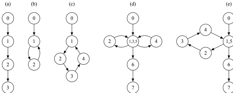
**Fig. 1** Sequence of iteration functions: (a) normal sequence. (b) fruitless 2-cycle. (c) fruitless 4-cycle. (d) two fruitless 2-cycles that end in normal sequence. (e) fruitless 4-cycle that ends in normal sequence.
