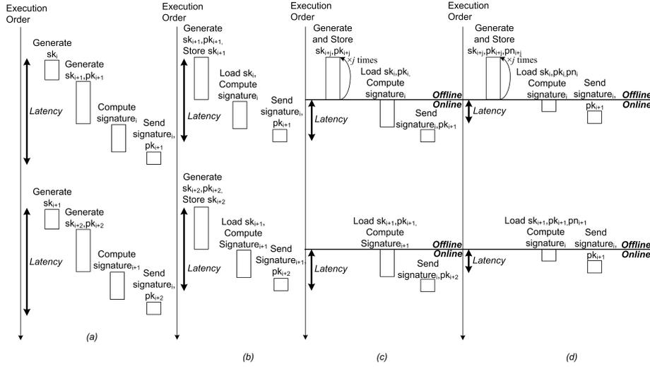
**Fig. 4.** Computation modes for (a) generic, (b) optimized, (c) partitioned, and (d) partitioned-with-precomputing execution
