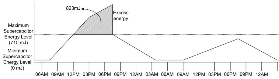
**Fig. 10.** The typical energy levels on the supercapacitor for two consecutive days (extrapolated from [8])
