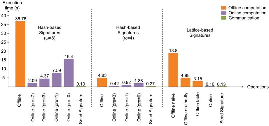
**Fig. 9.** The execution time measurements of signature schemes
