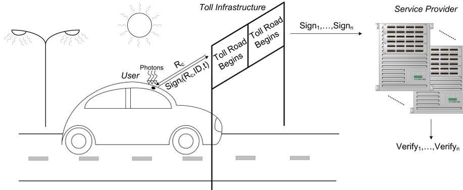
**Fig. 1.** The operations of a road tolling authentication system with digital signatures
