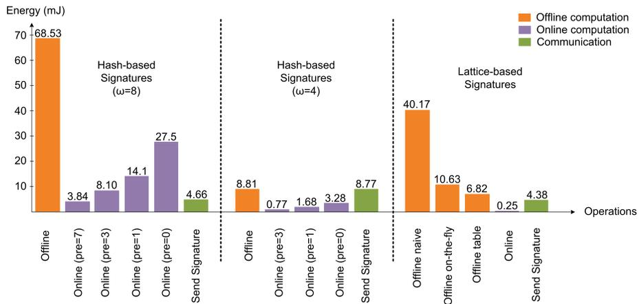
**Fig. 8.** The energy consumption measurements of signature schemes
