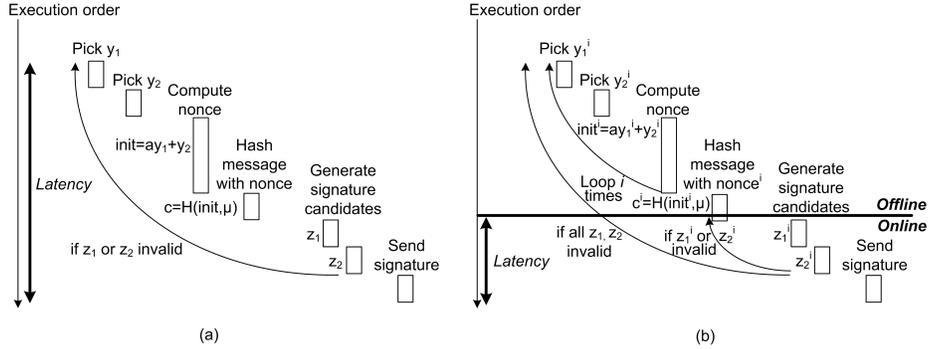
**Fig. 6.** Monolithic (a) and the partitioned (b) computation modes for the GLP signature scheme
