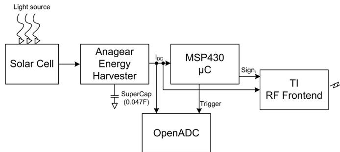
**Fig. 7.** The block diagram of the research platform
