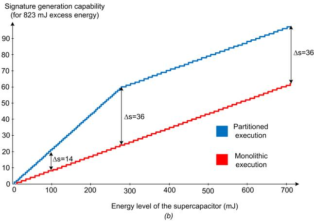
**Fig. 11.** Energy of the system vs. the total number of computable signatures for (a) hash-based and (b) lattice-based signatures
