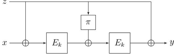
**Fig. 6.** The 3XSK[E] key-length extension scheme.
