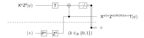
Figure 8: Functionality of the T-gate gadget.
