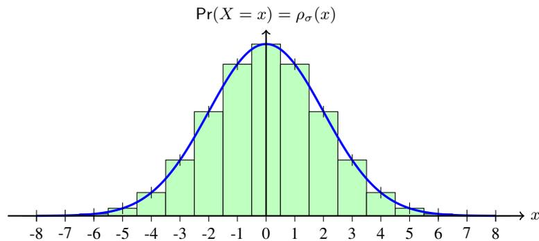
**Fig. 1.** The Discrete Gaussian distribution  $D_\sigma$  (Equation 3) is defined for all  $x \in \mathbb{Z}$  and satisfies  $\sum_{x=-\infty}^{\infty} \rho_\sigma(x) = 1$ . The green discrete bars illustrate the probability mass and the blue line is the corresponding continuous probability density function.
