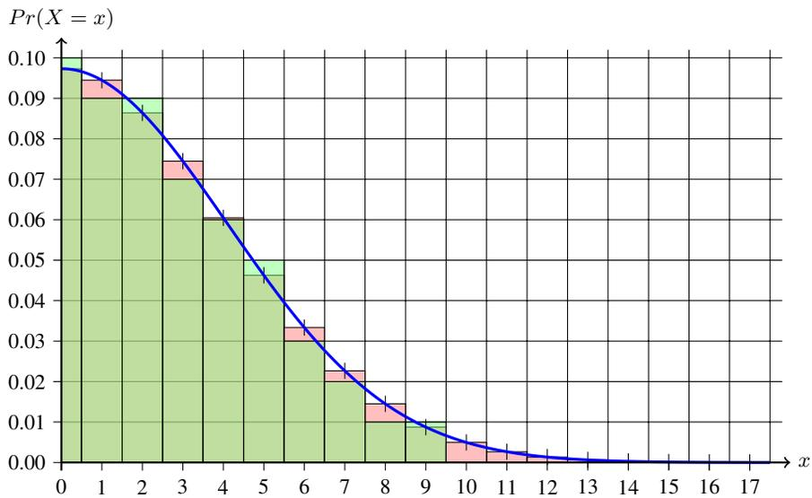
**Fig. 3.** Sampling the discrete Gaussian distribution with  $\sigma = 4.1$  and sampling precision 0.01. The red (rounded down) and green (rounded up) areas illustrate the statistical distance (total variation distance)  $\epsilon$  between the ideal distribution and sampling with the precision of the grid. Only the positive half  $x > 0$  of the symmetric distribution is shown. All  $|x| \geq 10$  are “tail”.
