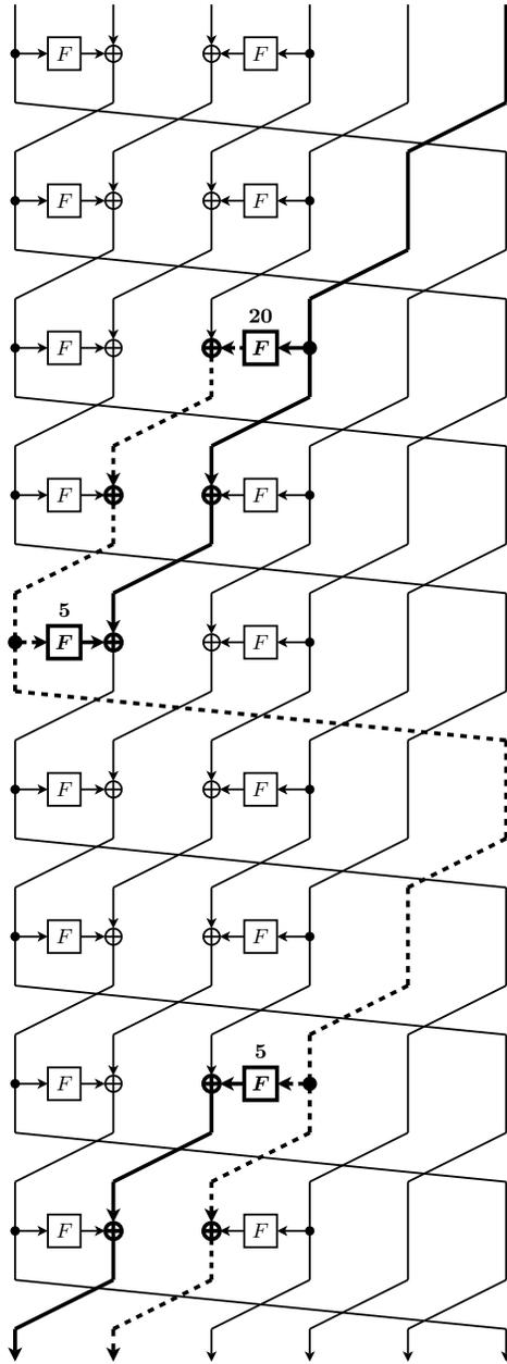
**Fig. 5.** A differential characteristic for  $b = 6$  with 30 active S-boxes. A thick full line indicates a difference in every byte, a thick dotted line refers to a difference in only one byte – it does not matter which one. A normal line indicates that no difference is present. When non-zero, the number of active S-boxes is shown above every  $F$ -function.
