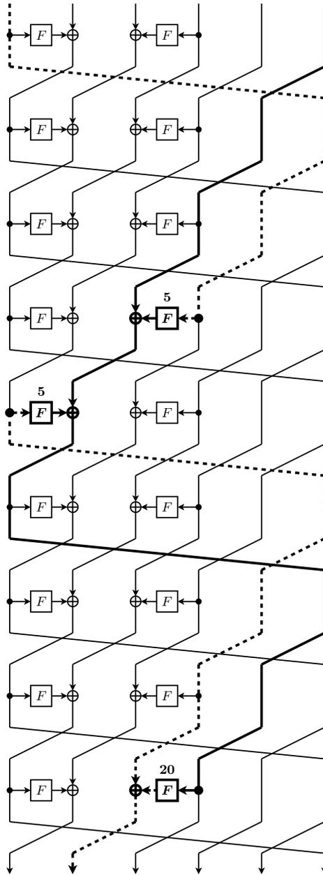
**Fig. 8.** Another linear characteristic for  $b = 6$  with 30 active S-boxes. A thick full line indicates a non-zero linear mask in every byte, a thick dotted line refers to a non-zero linear mask in only one byte – it does not matter which one. A normal line indicates that the linear masks of every byte are zero. When non-zero, the number of active S-boxes is shown above every  $F$ -function.
