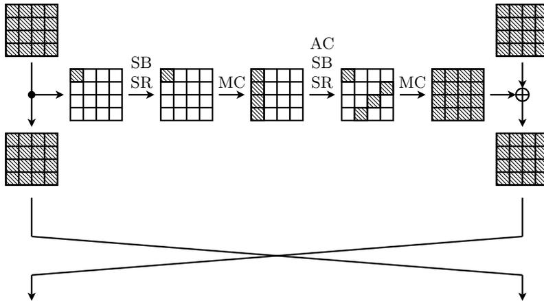
**Fig. 4.** A linear characteristic for one round of Simpira with  $b = 2$  with 5 active S-boxes. Crosshatches represent bytes with non-zero linear masks. As Simpira uses two AES rounds per  $F$ -function, it can reach 25 active S-boxes in only 5 Feistel rounds, corresponding to 10 AES rounds in total.
