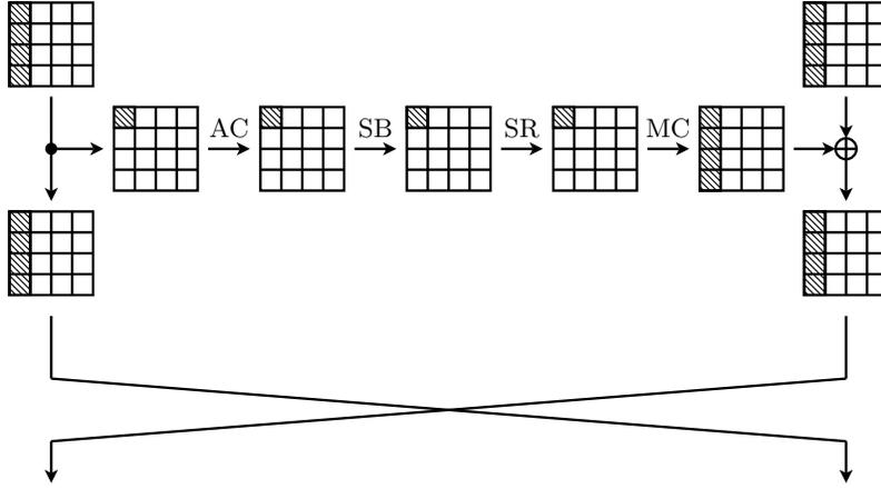
**Fig. 3.** A linear characteristic for an AES-based Feistel that uses only one round of AES inside its  $F$ -function. Crosshatches represent bytes with non-zero linear masks. The AES round consists of the **AddConstant** (AC), **SubBytes** (AC), **ShiftRows** (SR), and **MixColumns** (MC) operations. This round has only one active S-box. Therefore, 25 rounds are needed to ensure that there are least 25 linearly active S-boxes.
