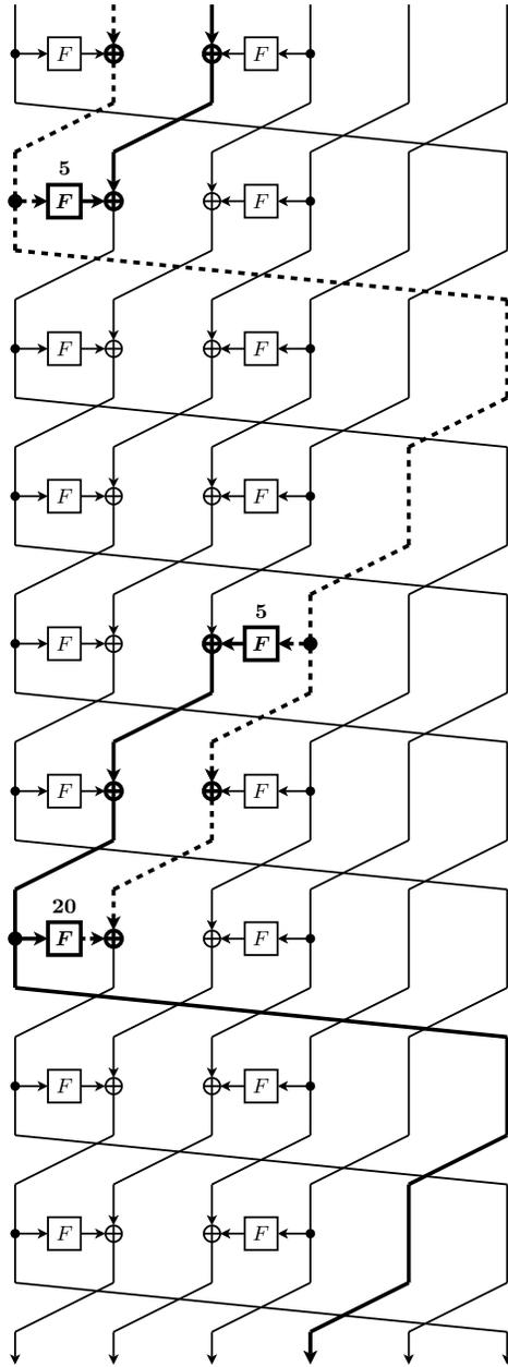
**Fig. 6.** Another differential characteristic for  $b = 6$  with 30 active S-boxes. A thick full line indicates a difference in every byte, a thick dotted line refers to a difference in only one byte – it does not matter which one. A normal line indicates that no difference is present. When non-zero, the number of active S-boxes is shown above every  $F$ -function.
