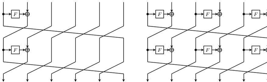
**Fig. 1.** Two common classes of Generalized Feistel Structures (GFSs) are the Type-1 GFS (left) and the Type-2 GFS (right). For each example, two rounds are shown of a GFS that operates on  $b = 6$  subblocks. We will consider these GFSs in this paper, as well as other GFSs with a different number of  $F$ -functions per round, and other *subblock shuffles* at the end of every round.
