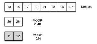
**Figure 2:** Queue state after 8 MODP 2048 exchanges. Numbers indicate generation order, and stale values are highlighted. If several connections have been made to the same DH group, the other DH group can grow stale as all nonces that were generated before those keys are used up.
