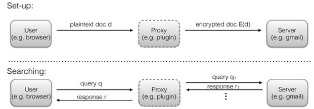
Figure 3: Architecture for a legacy-compliant SE scheme.
