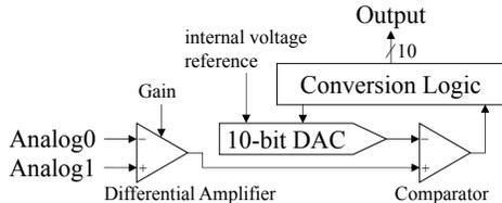
Fig. 6: Figure of the internal analog comparator.
