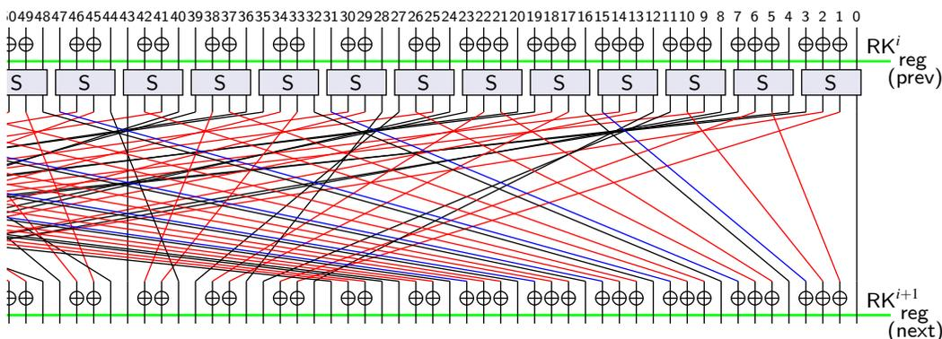
Fig. 10. A portion of the GIFT-128 round function. S is the GIFT S-box and  $RK_i$  is the  $i^{th}$  round-key. The state registers store the value corresponding to the position represented by the green horizontal lines.
