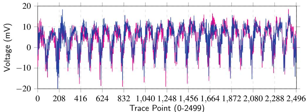
Fig. 14. **Power Trace:** Last 10 rounds of the protected GIFT implementation. The alternating big and small spikes correspond to the *state update* and the *intra S-box register update* respectively.
