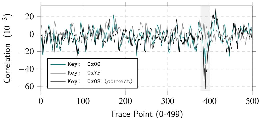
Fig. 12. **Correlation values vs. Trace Point:** For Key Byte 0. A large peak is visible only for the correct key  $0x08$ .
