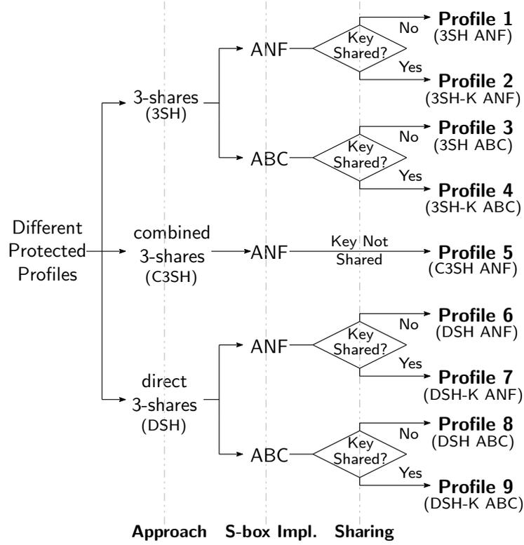
Fig. 5. Different Profiles for Threshold countermeasure
