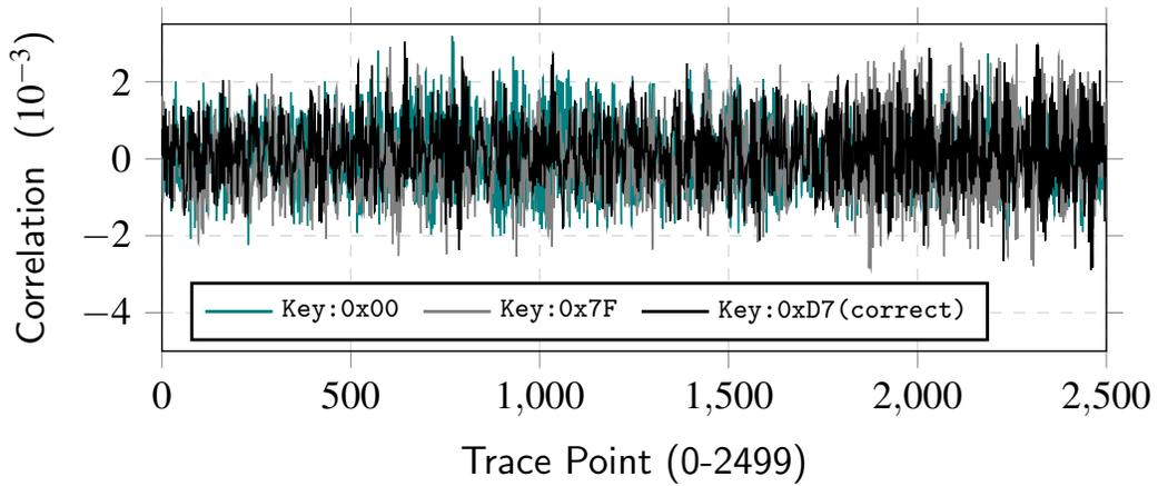
Fig. 16. **Correlation values vs. Trace Point:** The trace corresponding to correct key (0xD7) does not have any significant peaks, demonstrating the fact that CPA attack is unsuccessful.
