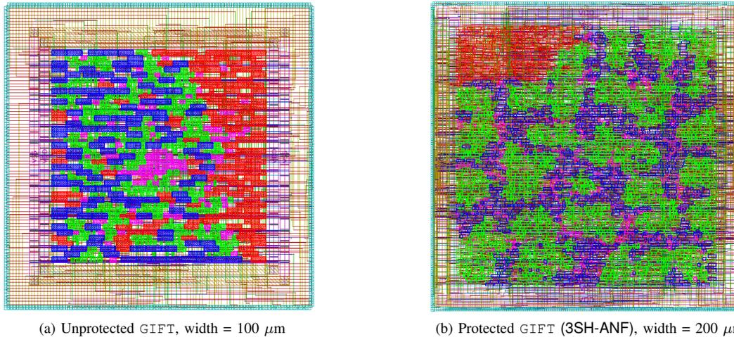
Fig. 7. Two of the *placed and routed* designs using *Synopsys IC Compiler*. Colors: S-reg (blue), Slayer (green), Key-reg (red), Glue Logic (magenta)
