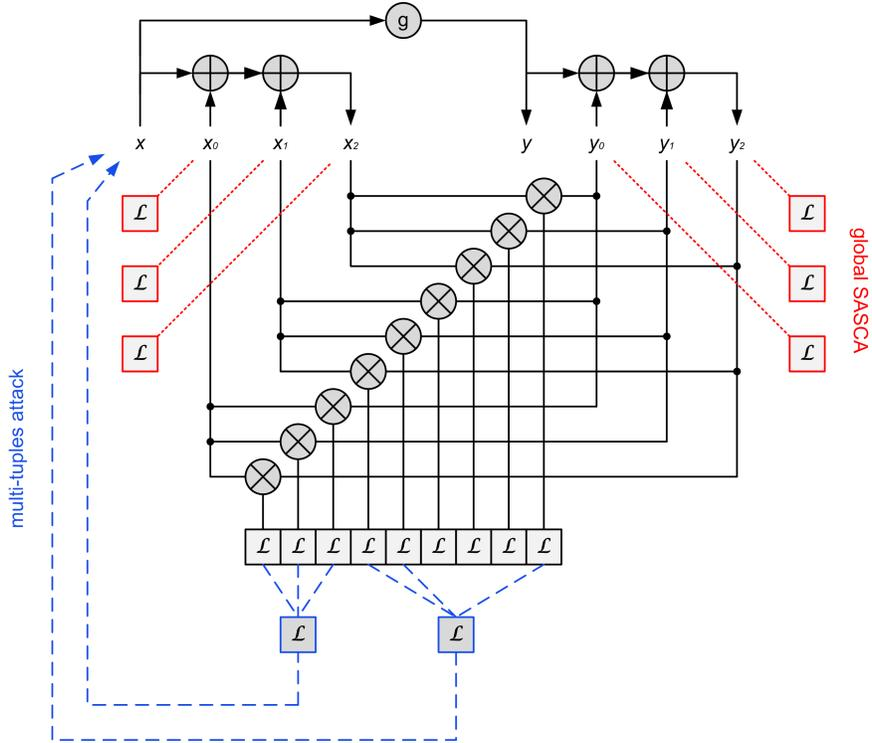
**Fig. 6.** Factor graph of a secure multiplication ( $d = 3$ ).
