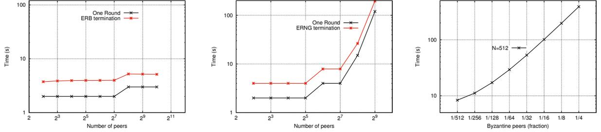
(a) Termination of ERB slightly increase with the number of peers. (b) Termination time of ERNG in function of the number of nodes in  $\mathcal{P}$ . (c) Time termination of ERB linearly increase with the number of byzantine nodes in  $\mathcal{P}$ .
