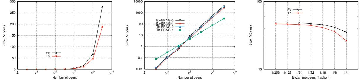
(a) Communication of ERB in function of the number of nodes in  $\mathcal{P}$ . (b) Communication of ERNG in function of the number of nodes in  $\mathcal{P}$ . (c) Communication of ERB in function of different byzantine peers in  $\mathcal{P}$ .
