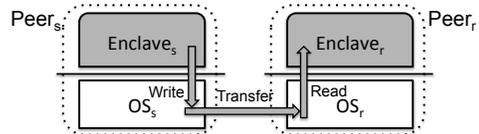
**Figure 1:** Each peer consists of two entities: an Enclave and an OS. The OS models the operating system and memory. The Enclave models the isolated memory and the secure execution of a program. The sender Enclave<sub>s</sub> can send a message via a secure channel to the receiver Enclave<sub>r</sub>. The grey areas are secure against malicious OSes of byzantine nodes.
