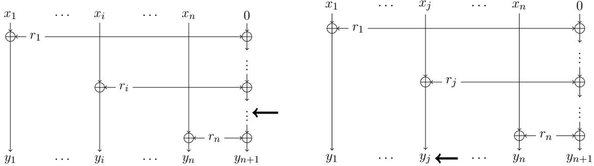
**Fig. 2.** Illustration of Lemma 5. Case 1 (left): the adversary has spent at least one probe on the last column for which  $x_{n+1} = 0$ , therefore we can have  $|I| \leq t - 1$ . Case 2 (right): no intermediate variable is probed on the last column; therefore  $r_j$  can play the role of a one-time pad for the simulation of the probed  $y_j$ , hence  $x_j$  is not required and again  $|I| \leq t - 1$ .
