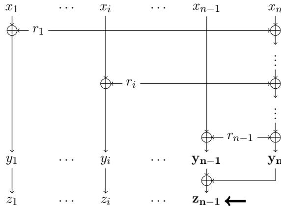
**Fig. 4.** Illustration of Lemma 8. If  $z_{n-1}$  is probed, then both  $y_{n-1}$  and  $y_n$  must be simulated, so we can apply Lemma 6 or Lemma 7 with probed  $y_n$ . If  $z_{n-1}$  is not probed, the simulation is straightforward, as in Lemma 2.
