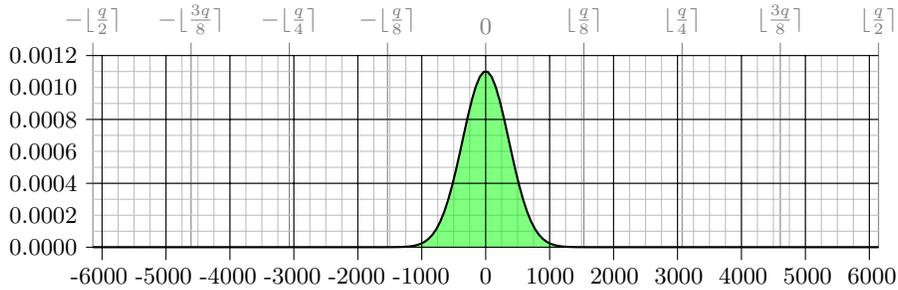
**Fig. 3.** The error distribution  $E$  of  $\delta = x_i - y_i$  (which we compute with high precision) is bell-shaped with variance  $\sigma^2 = 2^{17}$ . Its statistical distance to corresponding discrete Gaussian (with same  $\sigma$ ) is  $\approx 2^{-12.6}$ , which has a significant effect on the bit failure rate. This is why we compute the discrete distributions numerically.
