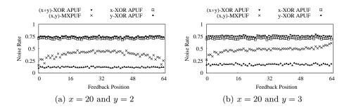
Fig. 3: Noise rate of (x+y)-XOR APUF, (x,y)-MXPUF, x-XOR APUF and y-XOR APUF when noise rate of APUF is around 0.05.
