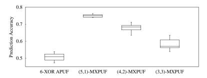
Fig. 4: Modeling of (x + y)-XOR APUF and (x, y)-MXPUF using CMA-ES and CRPs of PUFs. Each boxplot is built using 10 prediction accuracy values of 10 different models of a PUF design.
