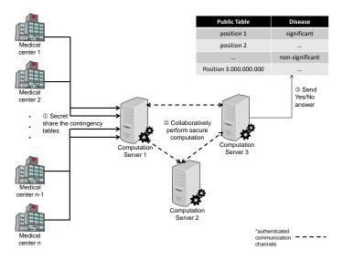
Fig. 2: A schematic representation of the multiparty computation scenario
