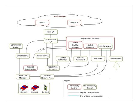
Figure 1: Overview of SCMS's architecture. Source:[12].
